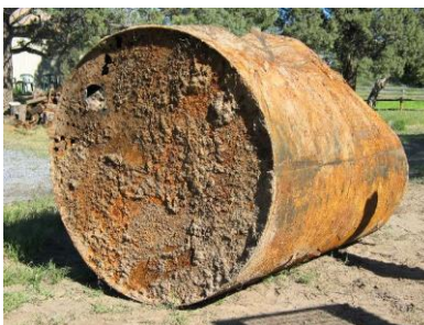
Rusted and leaking steel tank
