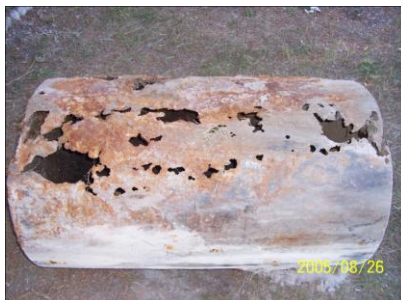
Rusted steel tank with large holes
